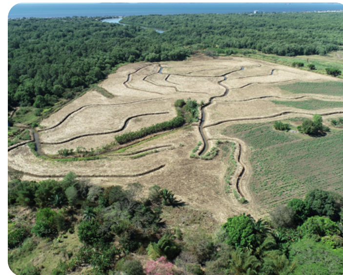
Since 2013, substantial losses of mangroves in Costa Rica's Gulf of Nicoya have been reversed through hydrological rehabilitation. Channels have been cleared and new channels created to allow tidal flows and natural mangrove regeneration, while enhancing ecosystem services and biodiversity. For further information, see: CATIE (in Spanish) © Danilo Torres Gómez, CATIE.
